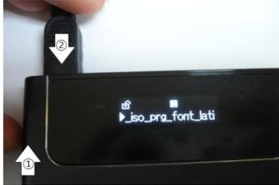
2. Press File Selection Switch in “End of List” until CD-MODE is shown. Then press button for 3 seconds to act as CD Mode.
