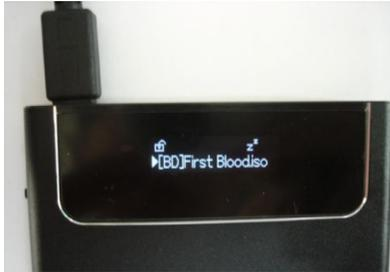
Power Save Mode enables longer OLED life by reducing the OLED brightness. It also puts the HDD into a Suspend Mode, which stops the HDD spin motor, resulting a less damage to the iodd hard disc as well as the connected PC and the port in case of accidental cable disconnection.
