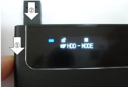
2. Press File Selection Switch in “Begin of List” until HDD-MODE is shown. Then press button for 3 seconds to act as HDD Mode.
